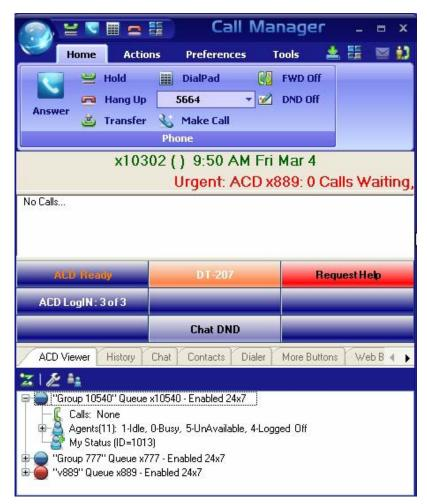
The ACD actions can be used to Log In / Log Out to/from ACD groups. Going temporarily unavailable and an ability to end wrap times can be part of the features available. Additional Call Center features are possible using User Programmable buttons.
